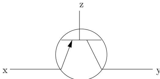
Figure 2.1: A schematic representation of a transistor.
