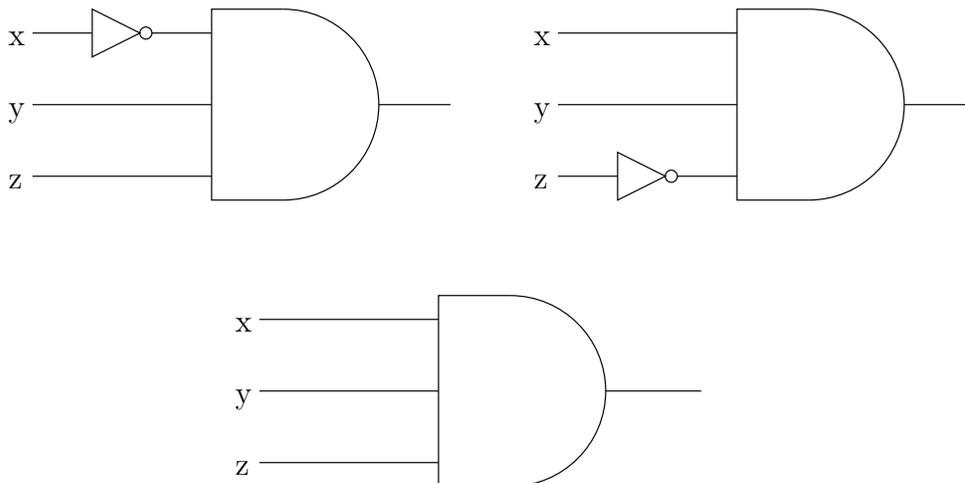
In Figure 2.5 we illustrate how to create a circuit whose i/o table is as above using these recognizers.
