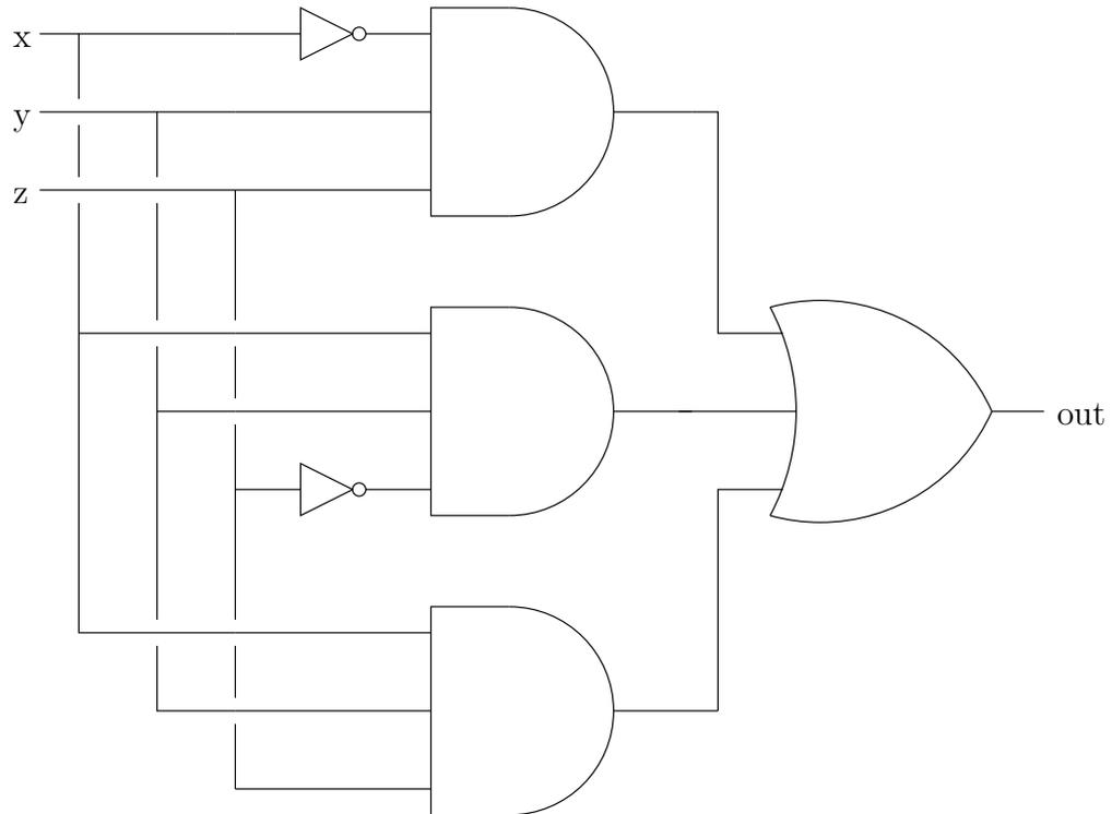
Figure 2.5: A digital logic circuit built using disjunctive normal form. The output of this circuit is  $(\neg x \wedge y \wedge z) \vee (x \wedge y \wedge \neg z) \vee (x \wedge y \wedge z)$ .
