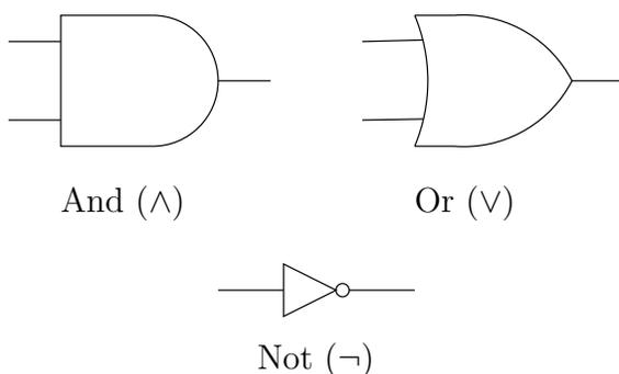
An and-gate has two transistors inside it that are wired in series – if both the inputs are energized the output will be too. An or-gate has two transistors in parallel inside it. Not-gates involve magic – when their input is not on, their output *is* and vice versa.
