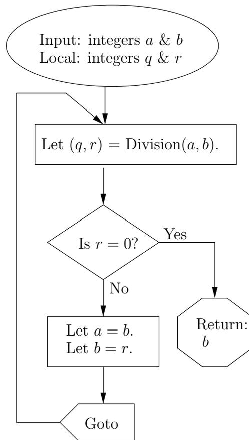
Figure 1.5: The Euclidean algorithm in flowchart form.
