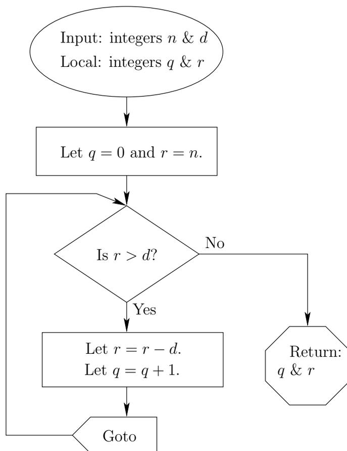
Figure 1.4: The division algorithm in flowchart form.
